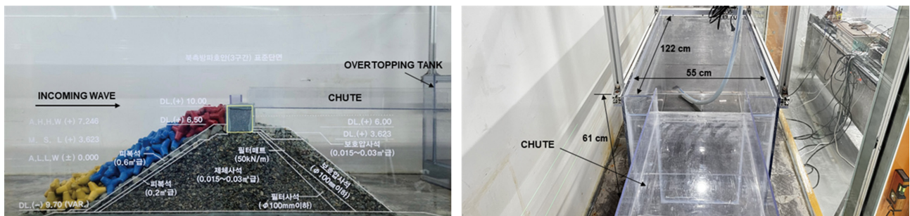
Fig. 4. Installation of the model structure and overtopping tank in the flume.
